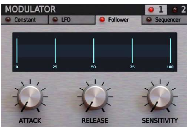
The Envelope Follower modulates the filter based on the amplitude envelope of the input signal
